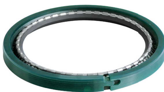
AIGI 5505HZ Duo-Lock Split and Wedge-shaped Cutting (Patented) NBR/FKM dynamic seal for high temperatures
